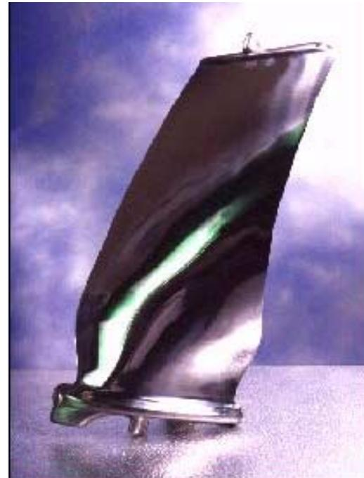
Figure 1. (a) An airfoil being removed from the die and (b) a large compressor blade made by precision forging.
