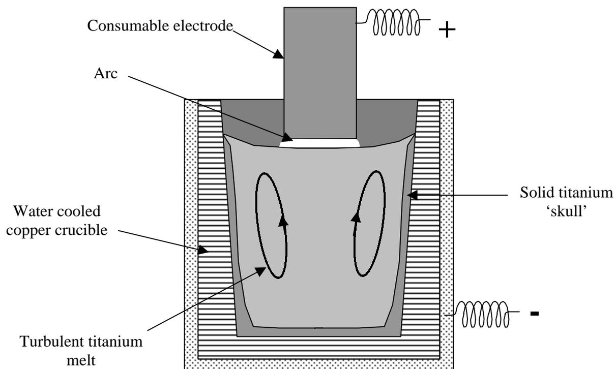
Figure 3. A schematic of the vacuum arc melting arrangement used for titanium casting. The arc is pulsed DC, this causes vigorous stirring and gives very good homogeneity.
