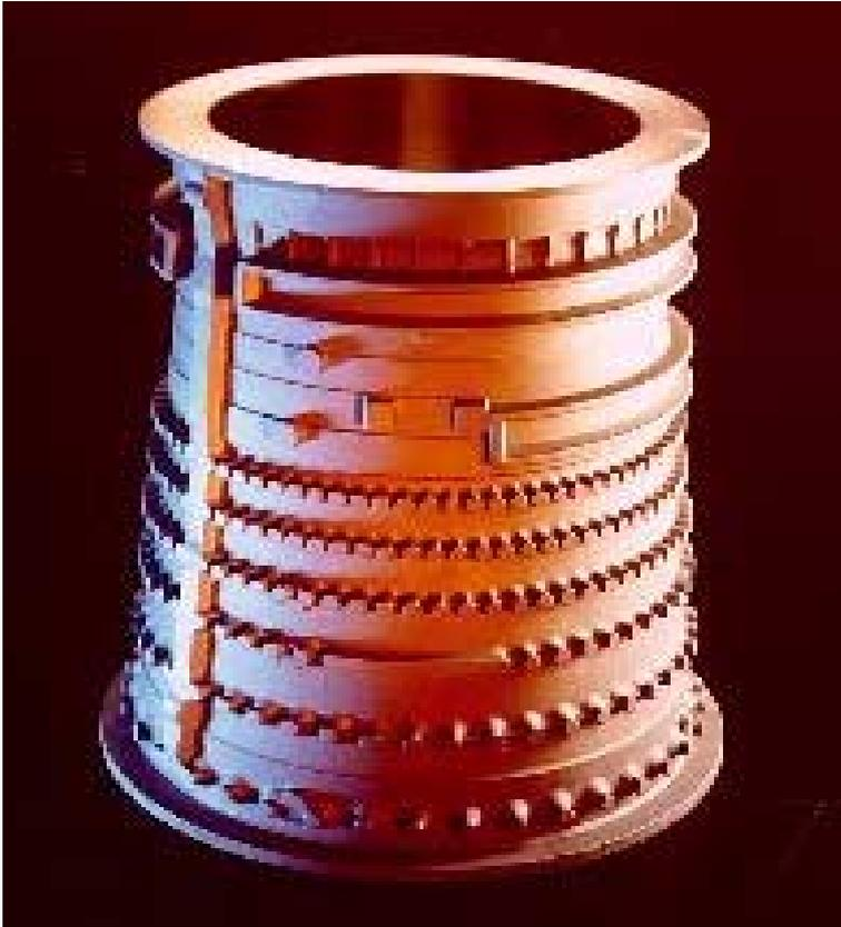
Figure 4. Titanium engine casing centrifugally cast into shell ceramic mould.
